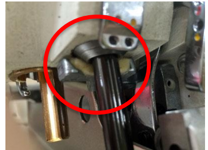
Needle bar oil suction system
