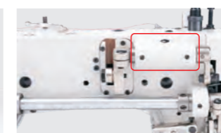
Sealed lifter shaft of presser foot
